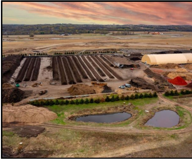
The current SMSC Organics Recycling site. Several windrows of organic material will be turned into compost. (Courtesy SMSC Organics Recycling Facility).
